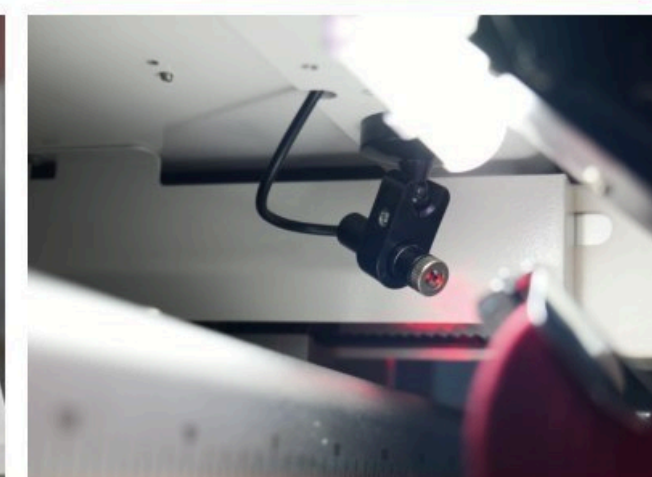
机头定位灯 Laser Positioning Light
