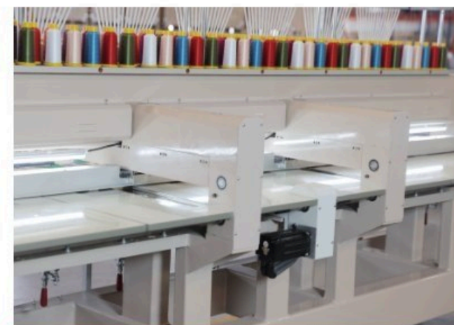
悬浮框架系统 Floating Driving System
