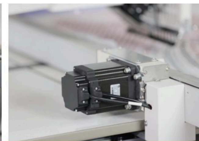
绣框采用高精度大电机 Precise Big Motors Make Accurate Frame Move
